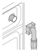
In order to prevent water leakage that may occur at the connection points, there are rubber seals (4) seals for the models with double water inlet and 2 seals for other models) attached to the hoses. These seals should be used at the tap and machine connection ends of the hoses. The plain end of the hose fitted with a filter must be attached to the tap and the elbowed end must be attached to the machine.
